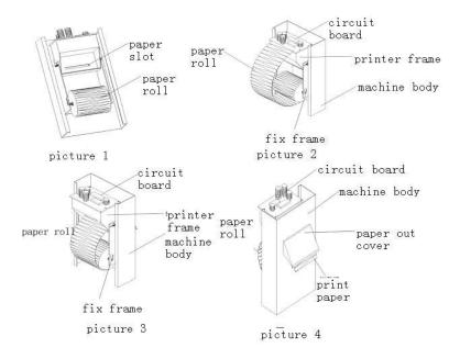
First: Make the axis threads the printing paper and fix them on the frame (picture 1)
