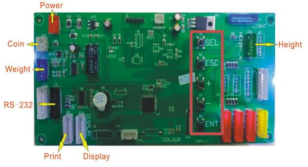
All functions are set and adjusted by keys on the main board (+ - SEL
