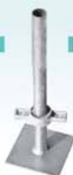
RFH-B011I 旋转调节底座 Swivel Adjustable Screw Jack Base 600 914mm Φ35/Φ38mm 150x150x8mm
