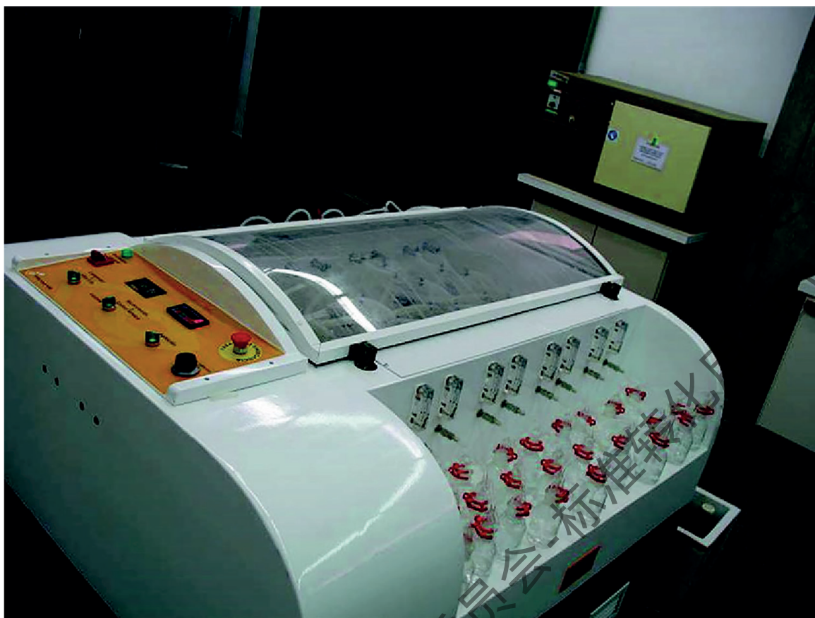
Figure A.1 — View of the unit for biodegradability assessment
