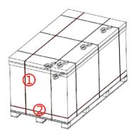
4. Cutting the carton and fold it down—Cut down the side of the carton by 1/2 to 2/3 height ( keep at least 1/3 height), then cut down the side of the carton (the folding line is about the red line in the figure) and cut off the four packing straps inside the carton.
