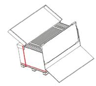
6. Cutting the remaining packing straps—When the remaining modules are covered by the uncut packing belt, two workers should hold the remaining modules, cut the no.1 packing belt and remove the top cover of the
