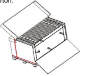
7. Remove remaining modules — When the remaining modules are covered by the uncut packing belt, two workers should hold the remaining modules, cut the no.1 packing belt and remove the top cover of the carton.
