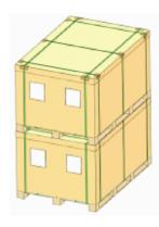
Cut off the whole packing belt of the pallet, and use a forklift to separate the two pallet modules.
