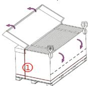
5. Taking out the modules in turn—Tear the tape from the first module border and remove the first module (make sure the remaining straps is tight to prevent the module from tipping). Tear off the tape on the frame in order of modules, and take out the remaining modules in order from the carton.
