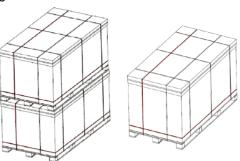
3. Openning the box cover—Open the box cover from that side where strap has been cuted. Turn the cover over to no. 1 strap.
