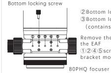
②Bottom locking screw ③Bottom load adjustment screw hole (contains M4 small screws) Remove the bottom lock screws when using
