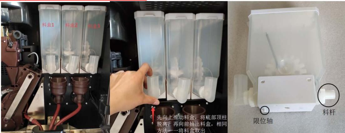
8.2.2.1 Open the main cabinet door (as shown in Figure 8-4), then push the box up with the discharge nozzle, make the limit column at the bottom of the box away from the sheet metal (as shown in Figure 8-5), then pull the box forward, and take out the box one by one in the same method (as shown in Figure 8-6). From left to right is 8-4, 8-5, 8-6
