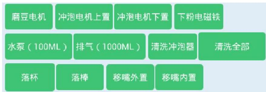
6 After standing, then click the exhaust 1000ml 2-3 times. This cleaning is easy to discharge the water scale dissolved in the water pipe.
