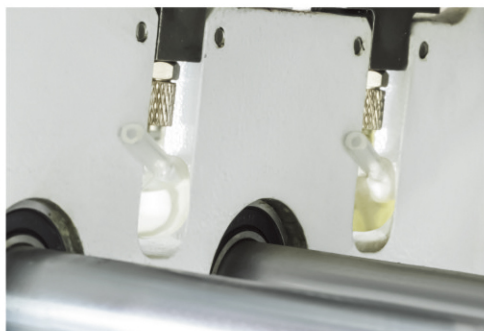
独特的油囊供油系统 (专利结构) Unique oil bag oil supply system (Patented structure)
