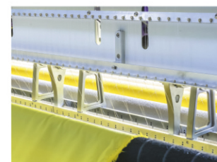
铝合金针、压杆架 Aluminum alloy needle and pressure rod holder
