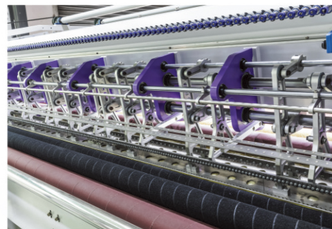
铝合金针、压杆架 Aluminum alloy needle and pressure rod holder
