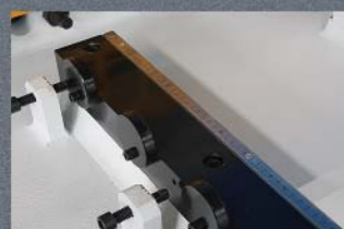
垂直度调整及前定位 Vertical Adjustment And Front Stop Position Device
