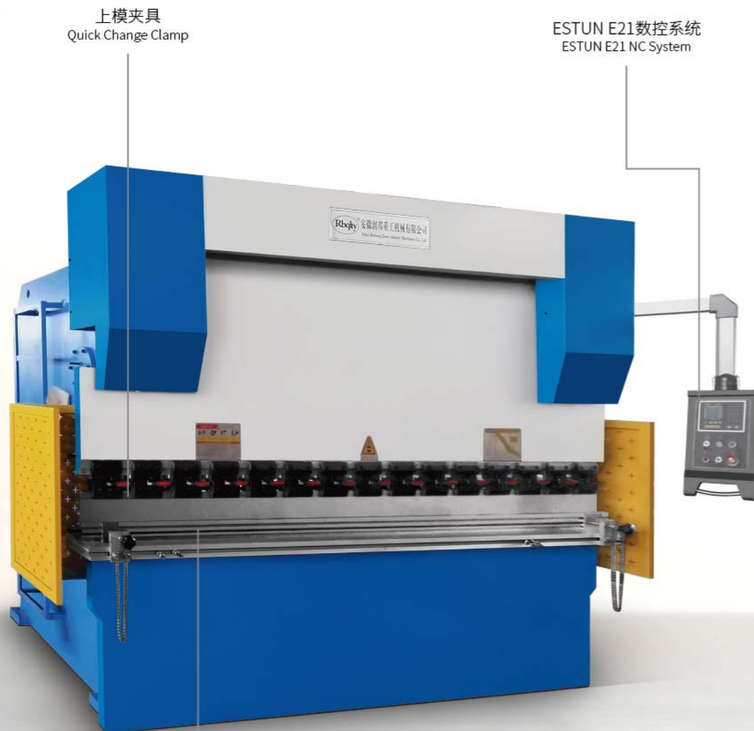
42CrMo折弯机模具 42CrMo Press Brake Tooling
