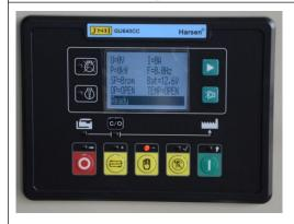
Standard control panel can satisfy the Genset for normal operation, it have the advantages of simple operation, multiple functions, reliable protection. The panel can receive remote open/stop control signal for Genset. (ATS control)
