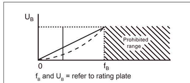
If this is ignored, the motor current will increase disproportionately and the drive motor will fail to achieve its rated speed.
