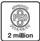
Additionally, the majority of HYSON springs are **PED** (Pressure Equipment Directive) approved to withstand a minimum of 2 million full cycles according to PED (2014/68/EU). Many of our competitors are in compliance of PED, but compliance is unequal to the 2 million cycle test and approval that HYSON gas springs have undergone. This is one more assurance that with HYSON Nitrogen Gas Springs, you receive an added value of reliability and operational excellence.
