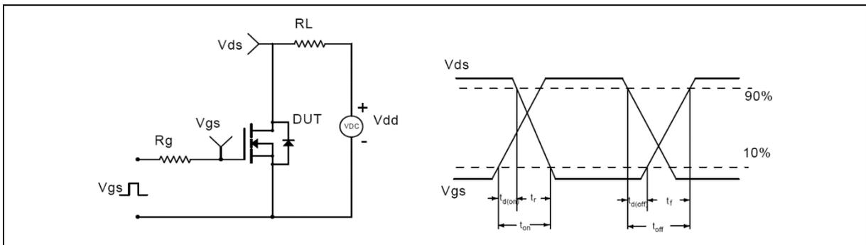
**Figure 2. Switching time test circuit & waveforms**
