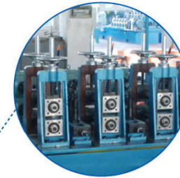
Needle Bearings in operation side Horizontal Stand, easier and faster to change the Roll Sets
