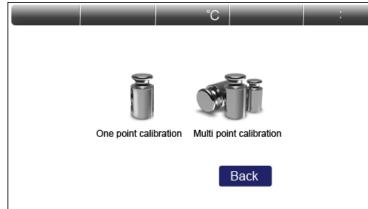
When the instrument error or improper operate. Calibration weights can be adjusted with accuracy.Press "One point calibration" and does not release until it display"-cal-",Then flashing put on the "100.000", put on the calibration weight, then it will display "= = = = = ", until it display "100.000", and will show remove the weight, it will display "= = = = = "again, Waiting it show" 0.000 ", the calibration is completed.
