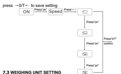
Keep pressing  $\mathbf{ON},$  when  $\mathbf{Unit}$  is shown ,Then operation as blow:
