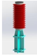
Figure 7 Installation of double magnetic separation bracket
