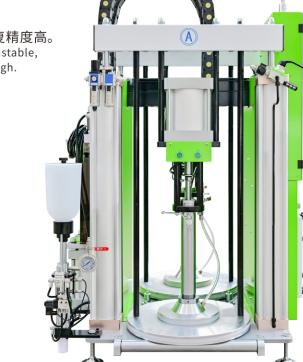
专利截止阀、气动射嘴。 Patent cut-off valve, pneumatic nozzle.
