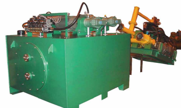
74MN平板硫化机液压系统 74MN hydraulic system for flat vulcanizing machine
