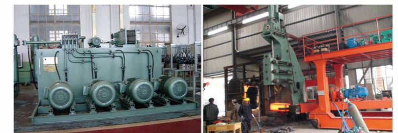
电液锤液压系统及应用现场/Application of hydraulic system for electro-hydraulic forging hammer
