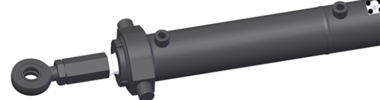
Steering hydraulic cylinder FAST Standard code: ZBJ-ZXφ63/32-215 Specification: 63/32X215-170 Qty: 2
