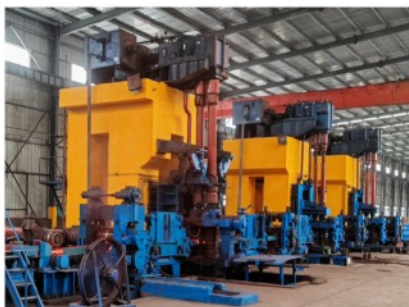
Horizontal And Vertical Finishing Mill Unit
