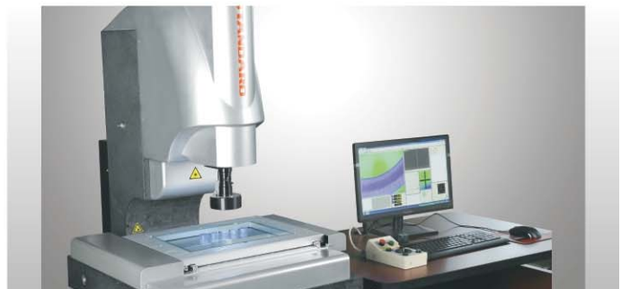
全自动二次元投影仪 Accurate Size Test Equipment 测量精度5 \mu m, 放大倍率18X-120X
