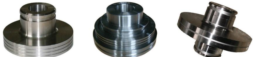
Plate & Snap Ring, Plate material used is ASTM1020 steel, Material of snap used is ASTM1066 steel. it is divided into A、K、B、L type.
