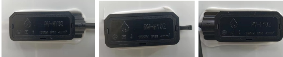
Fig. 3: View of junction box of module type ESPHSC440
