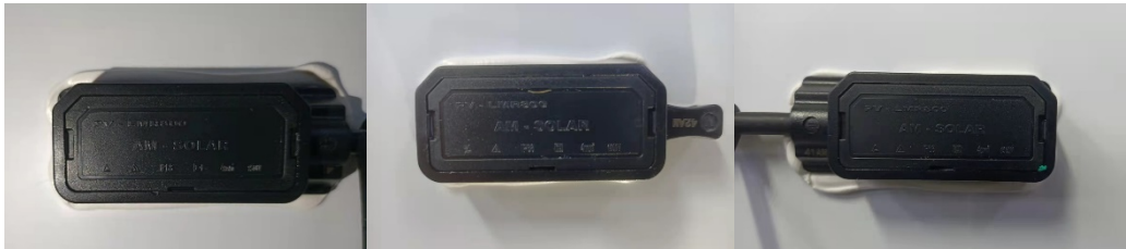
Fig. 3: View of junction box of module type ESPHSC550
