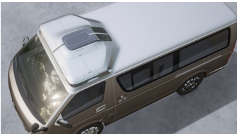
L4 level autonomous driving Rooftop sensor fusion unit
