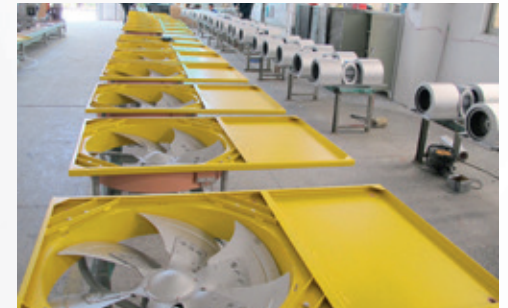
9. Product Testing - Inspected for dimensional integrity, tested for vibration, noise, energy usage etc. Packaged after passing inspection
